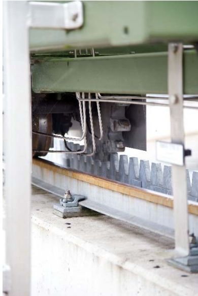
Rail wheel with gear drive
