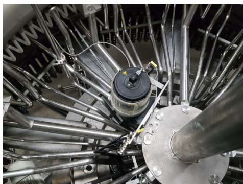
Fig. 1: Filler carousel with central lubrication and progressive feeder
