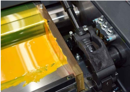
Lubrication of roller bearings and side jaw ink fountain with ELKALUB GLS 964/N2
