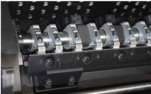
Gripper seat lubrication with ELKALUB FLC 4010
