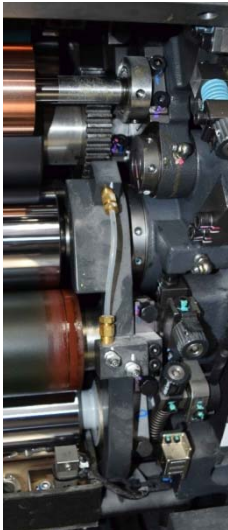
Lubrication of bearings and gear wheels in the inking/dampening unit with ELKALUB GLS 964/N2
